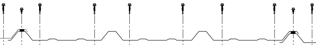
PBR-Panel Fastening Pattern - Ends
