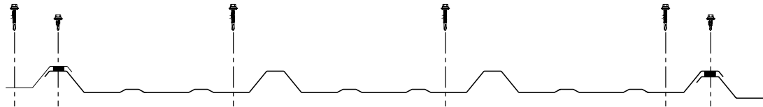
R-Panel Fastening Pattern - Interior
